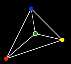
$$\alpha = \frac{Area(\mathbf{CC_{1}C_{2}})}{Area(\mathbf{C_{0}C_{1}C_{2}})}$$
