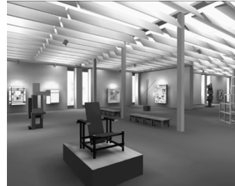
Museum simulation. Program of Computer Graphics, Cornell University. 50,000 patches. Note indirect lighting from ceiling.
